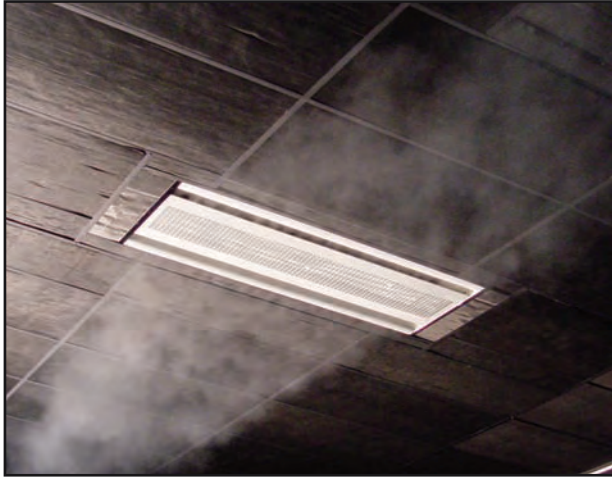
Air flow tests in R&D-Innovation laboratory
