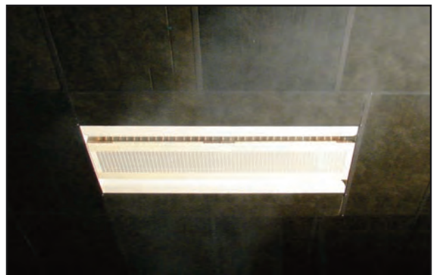
Laboratory test. 45° deviation of the air jet
