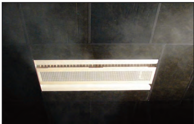
Laboratory test. V-shaped air jet orientation
